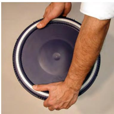
3. Rotate the lid firmly 90 degrees in a clockwise direction to close on the quarter turn threads. This can be done in one operation. Press downwards while rotating the lid until the lid locates over the button. Listen for a click as the lid passes over the button. The lid is now closed.
